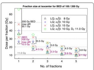
**Fig. 4** Fraction dose necessary to deliver a BED equal to 100 and 200 Gy under the assumptions of the LQ model with  $\alpha/\beta$  of 8, 10, and 15 Gy and LQ-L model with  $\alpha/\beta$  equal to 10 Gy and a D<sub>t</sub> value of 11.0 Gy, estimated for doses at the isocenter
