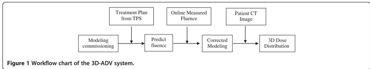
**Figure 1** Workflow chart of the 3D-ADV system.
