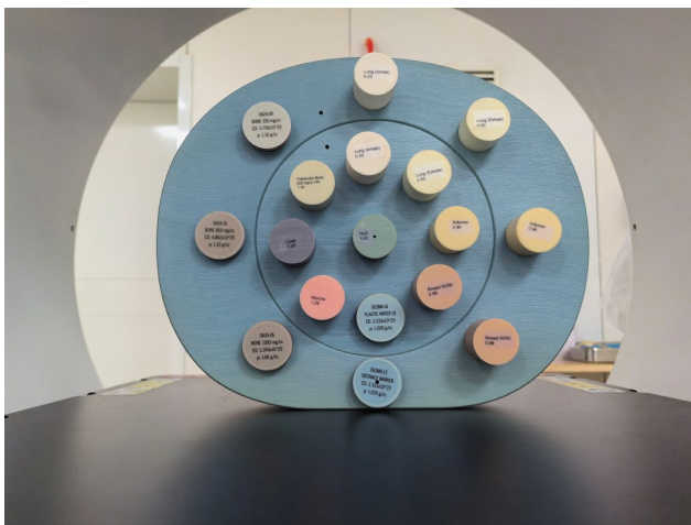
Fig. 1 Insert arrangements of 062 M phantom for measurements of the accuracy of the relative ED value
