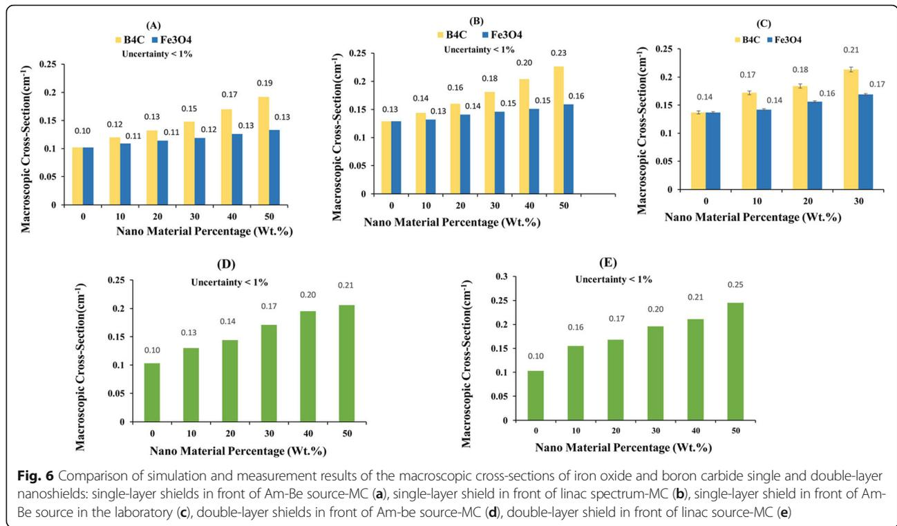
**Fig. 6** Comparison of simulation and measurement results of the macroscopic cross-sections of iron oxide and boron carbide single and double-layer nanoshields: single-layer shields in front of Am-Be source-MC (a), single-layer shield in front of linac spectrum-MC (b), single-layer shield in front of Am-Be source in the laboratory (c), double-layer shields in front of Am-be source-MC (d), double-layer shield in front of linac source-MC (e)
