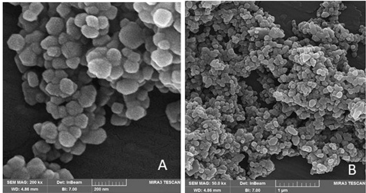
**Fig. 3** Scanning electron micrograph of NPs from Iranian Nanomaterials Pioneers Company, NANOSANY; iron oxide NPs (a), boron carbide NPs (b)
