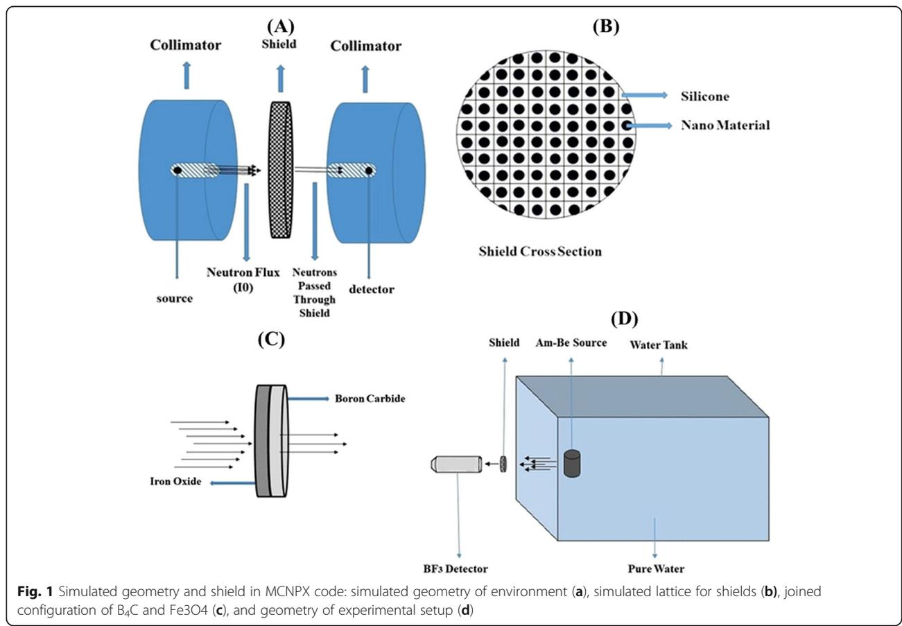
**Fig. 1** Simulated geometry and shield in MCNPX code: simulated geometry of environment (a), simulated lattice for shields (b), joined configuration of B<sub>4</sub>C and Fe<sub>3</sub>O<sub>4</sub> (c), and geometry of experimental setup (d)
