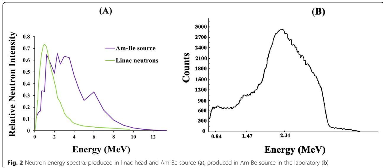
**Fig. 2** Neutron energy spectra: produced in linac head and Am-Be source (a), produced in Am-Be source in the laboratory (b)
