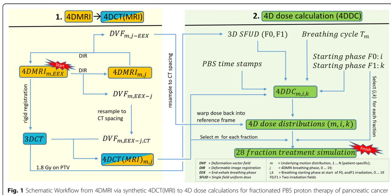
**Fig. 1** Schematic Workflow from 4DMRI via synthetic 4DCT(MRI) to 4D dose calculations for fractionated PBS proton therapy of pancreatic cancer
