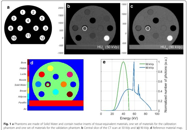
e 50 kVp and 90 kVp photon spectra used for SECT and DECT
