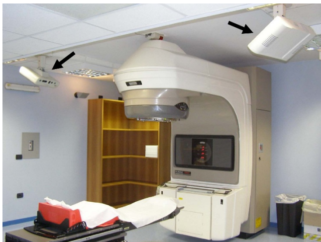
Figure 1 Photograph of the two camera pods (black arrows) of the surface registration system, mounted on the ceiling of the treatment room. The linear accelerator is also shown.
