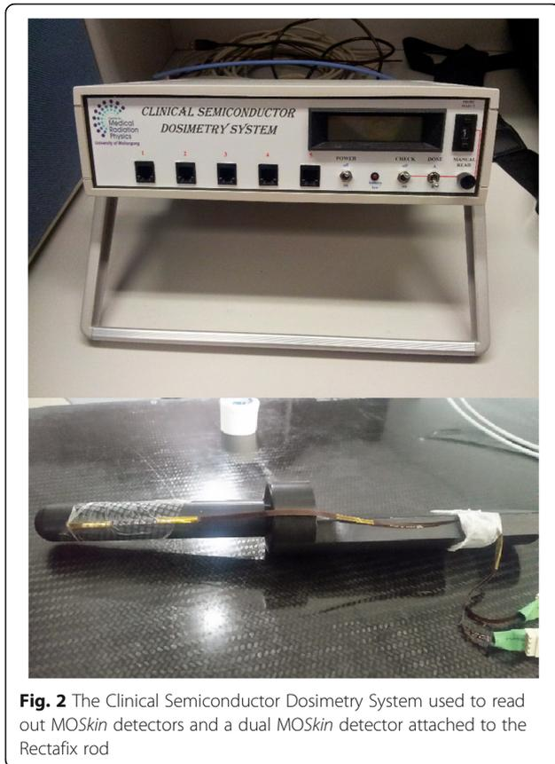
**Fig. 2** The Clinical Semiconductor Dosimetry System used to read out MOSkin detectors and a dual MOSkin detector attached to the Rectafix rod
