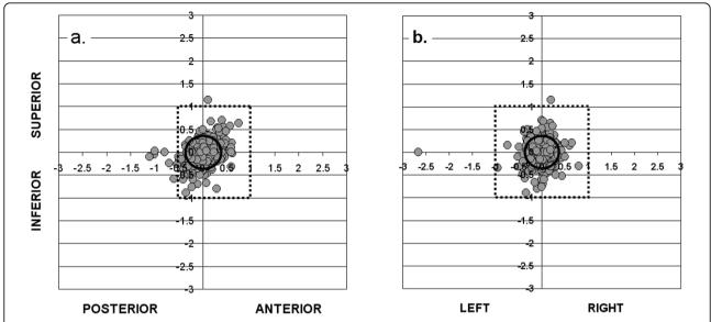
Figure 2 Isocenter placement errors (in cm) relative to DRR on during-treatment EPIs (gray circles; n = 530 fractions), along a): S-I and A-P axes, and b): S-I and L-R axes. Outer box shows PTV margins used in the study; inner ellipse shows 95% confidence intervals for CTV coverage in each direction.
